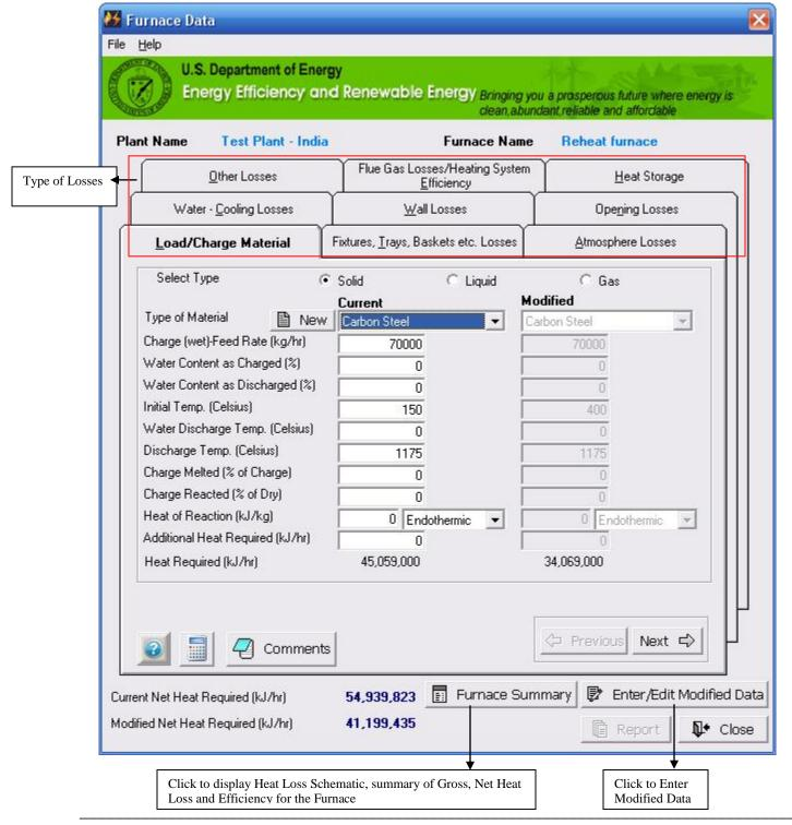
There are nine tabs that represent commonly encountered losses (mentioned below) in a furnace. The screens are designed for use with fuel fired furnaces but can also be used for electrically heated (i.e.
