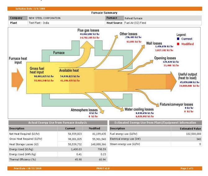
Note: The diagram shown above is a "Static Sankey" diagram.
