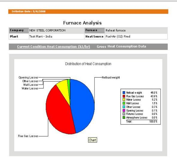
HeatStorage (kJ): 90,152,929 Thermal Efficiency (%): 45.98 Area of Heat Consumption kJ/hr Netload weight 45, 059, 000 Flue Gas Losses 43,062,002 Water Losses 8,038,656 Wall Losses 1,456,656 Other Losses 256,483 Opening Losses 129,028 Fixtures Losses 0 Atmosphere Losses 0 98 001 825
