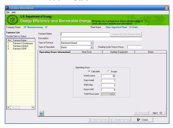
To start with, enter furnace name (mandatory), description and select type of furnace and operation. If the furnace operates in a batch mode, enter the heating cycle time (mandatory).
