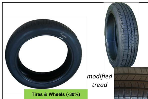
Figure V-12: Photographs of tall/narrow prototype tire.
