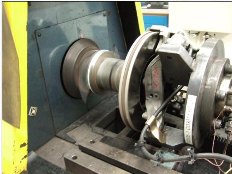
Figure V-11: Aluminum brake under test.
