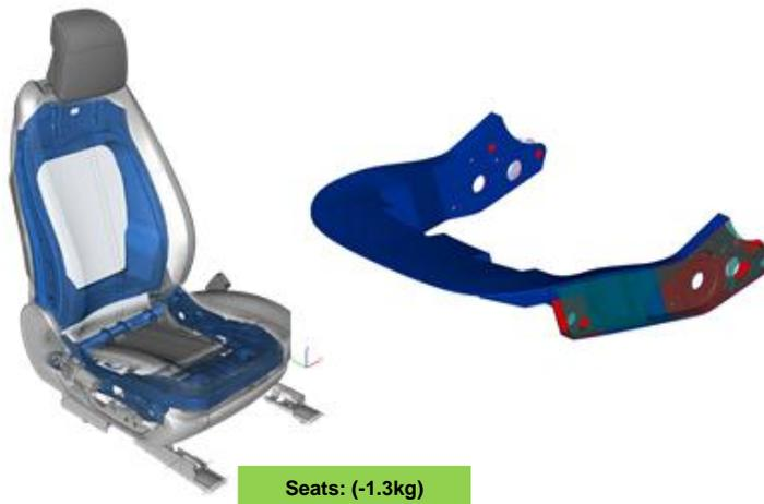
Figure V-9: Carbon Fiber seat back and cushion structures.
