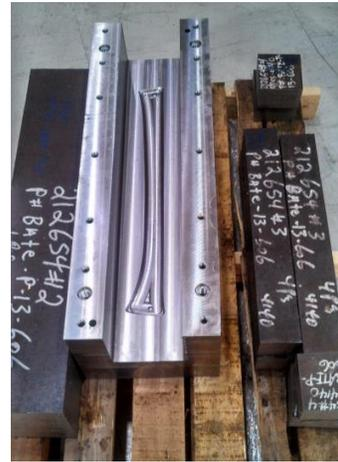
Figure III-38: Views of forming tools during fabrication at Magna SCFI.
