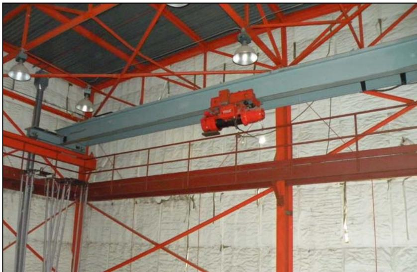
Figure 2-3. Crane and trolley shown above the catwalk
