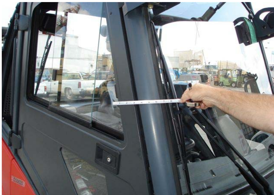
Figure 2.3-2. Linde Forklift Depicting Field of View Impairment
