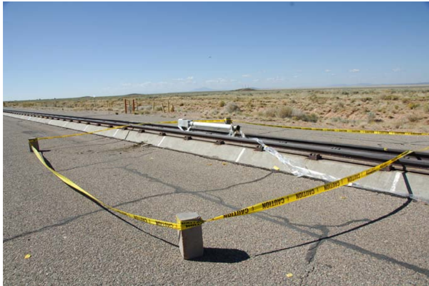
Figure 2-2. Position of rocket and test package after accident
