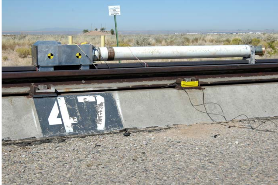
Figure 2-1. Representative rocket motor and test package
