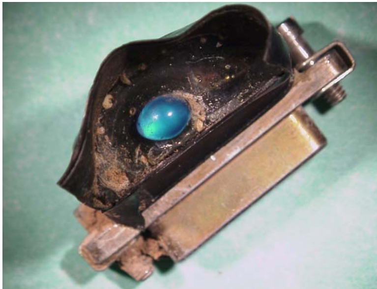
Figure 2-5. Post accident LED module with black electrical tape
