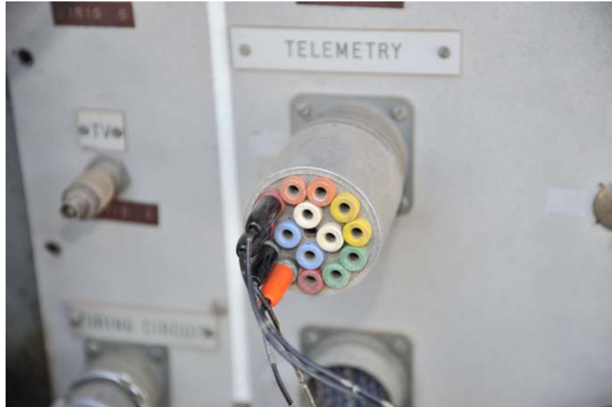
Figure 2-7. HiCapPen connection to sled track side box
