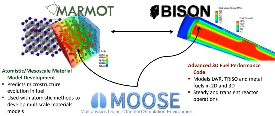
Simulation framework allowing rapid development of FEM-based applications
