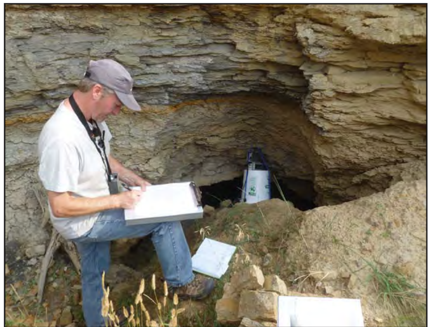
An LM contractor collects radon measurements at the mouth of an adit in the Little Ann Mine in the Edgemont District in South Dakota during a field visit.
