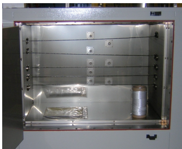
Figure 3. Five-pass oxidation oven.
