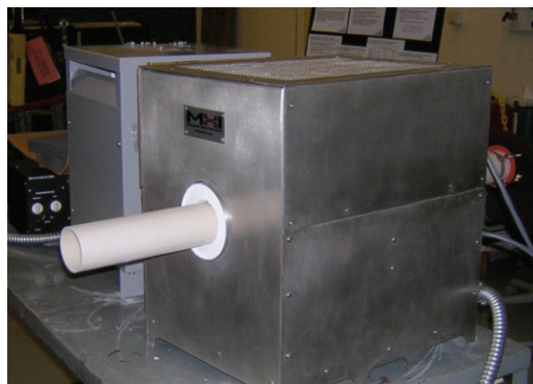
Figure 2. 1750°C carbonization furnace.
