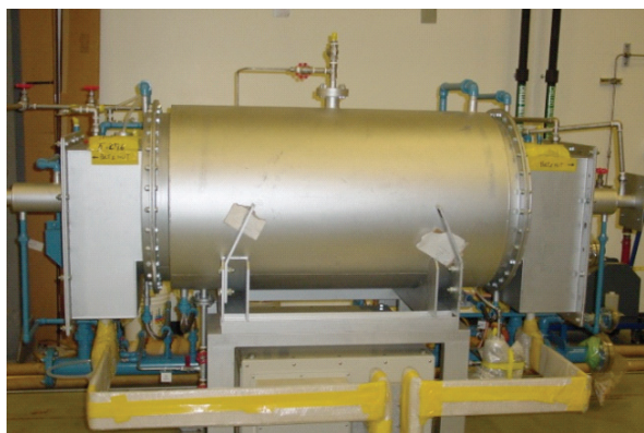
Figure 1. 2500°C graphite tube furnace.
