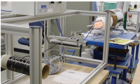
Figure 6. Processing of FISIFE precursor using ORNL's precursor evaluation line.
