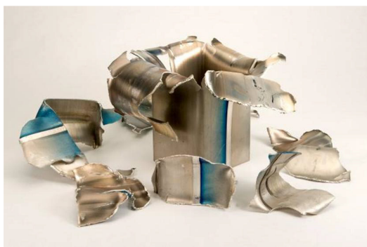
Figure 4. Final deformed shape of the extruded Mg AM30 beam after an axial compression test.
