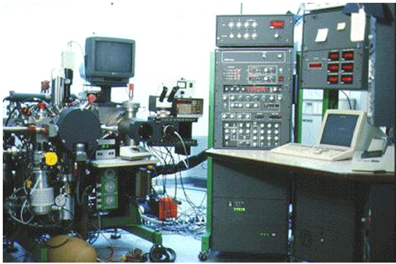
Figure 2. ORNL Cameca IMS 4f SIMS system currently being upgraded for rapid isotopic ratio diffusion depth-profile measurements.
