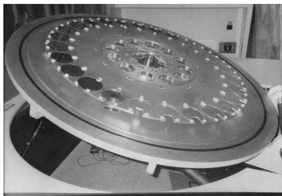
Figure V - 177: Opened specimen handling target chamber, denoted as a wafer handler. In this photograph several 10 cm specimens for demonstration are shown in specimen positions.
