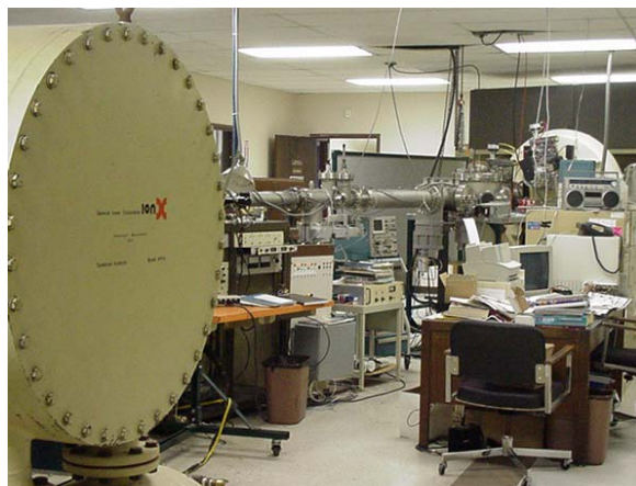
Figure V - 176: UES, Inc. Tandatron. The accelerator tank is in the foreground and the specimen target chamber is the disk shaped object partially visible at the end of the beamline.
