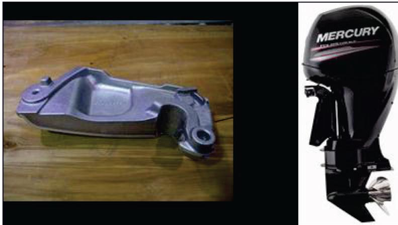
Figure 9. Mercury Marine Transom Bracket Cast by the Ablation Process
