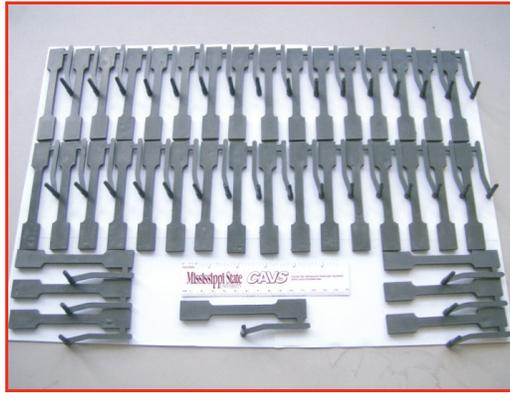
Figure 10. Molding trial by Ti alloy feedstock.
