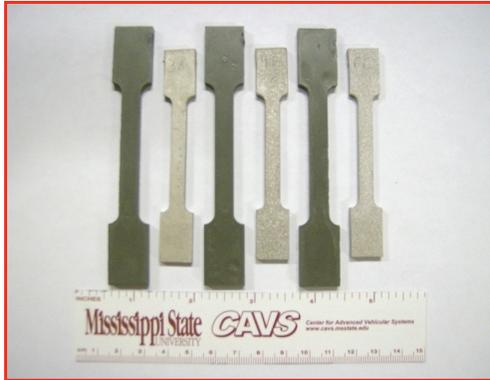
Figure 14. Green and sintered PIM parts arranged alternately.
