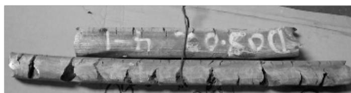
Figure 5. Excessive Cracking Encountered in the Initial Rolling Trials of the Ti64 (top) and Ti5553 (bottom) Alloys
