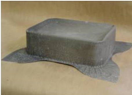
Figure 14. Rectangular pan formed to full depth from DC-Cast AZ31.
