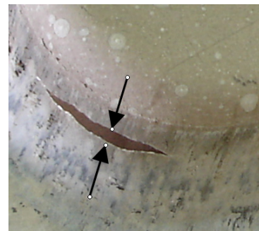
Figure 19. An example of a corner split measured for the estimation of pan depth.
