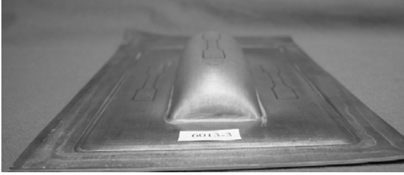
Figure 1. Superplastically-formed tray to be used as evaluation part for the high SPF alloy development project.
