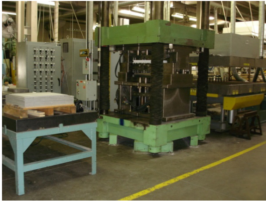
Figure 16. Photograph of new dedicated press and pre-heater for the development of the fully automated warm-forming cell.
