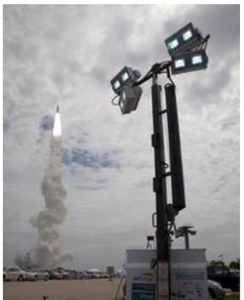
Hydrogen fuel cell powered light tower at Space Shuttle launch
