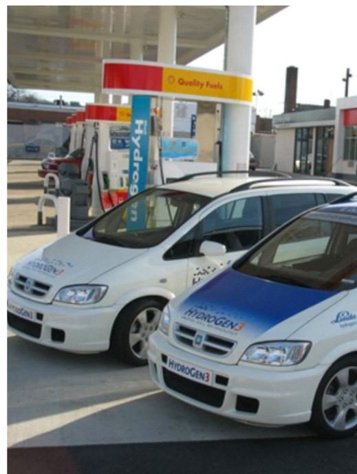
The hydrogen dispenser at this Shell station in Washington, D.C. offers both gaseous and liquid hydrogen.
