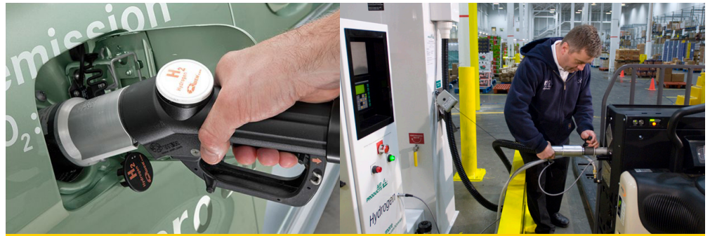
Like natural gas vehicles, hydrogen vehicles and hydrogen fuel cell material handling equipment are refueled using a closed-loop system that helps to ensure safe operation.
