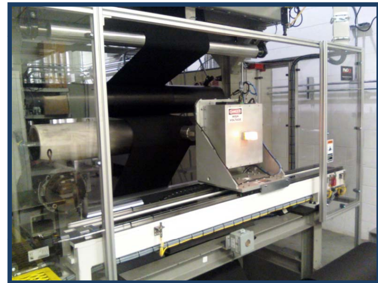
This is the first time a scanning XRF has been used on GDEs – BASF
