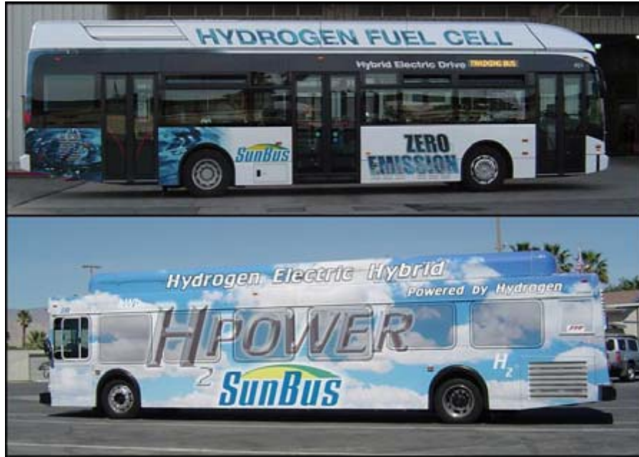
Figure 2. Fuel cell (top) and HHICE (bottom) transit buses at SunLine
