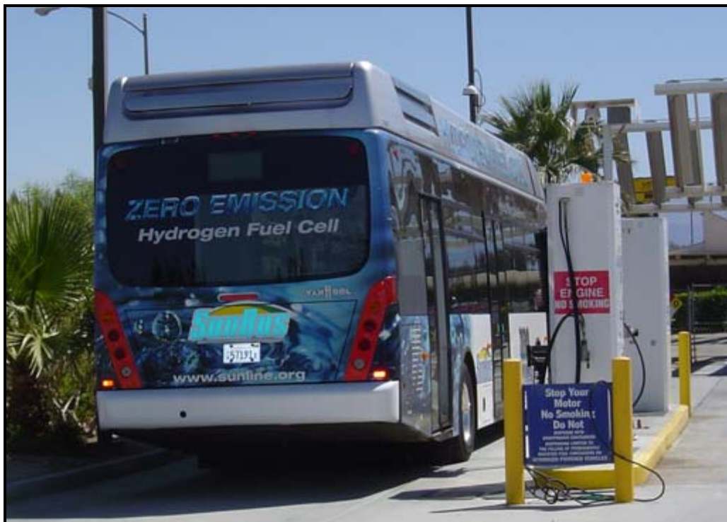
Figure 5. SunLine's fuel cell bus during fueling
