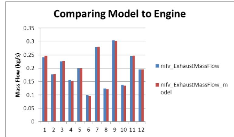
Figure 52 Comparison of Engine Exhaust Mass Flow versus Model Output
