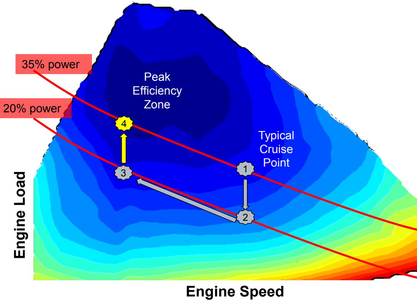
Analysis of typical diesel engine efficiency profile.
