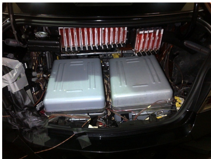
TED heat exchanger/controller/data logger in the trunk of LaCrosse
