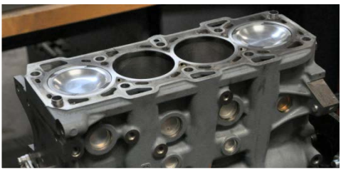
Modified RCCI pistons installed in GM 1.9-L diesel engine
