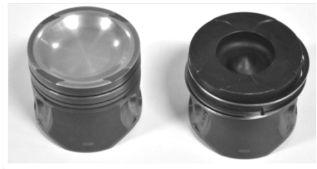
RCCI Optimized (left) and OEM (right) pistons
