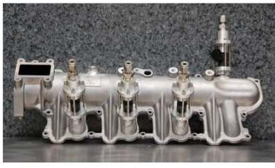
Modified Intake Manifold with PFI Injectors
