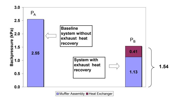
Whether backpressure would go up , go down, or stay the same depends on the heat exchanger design
