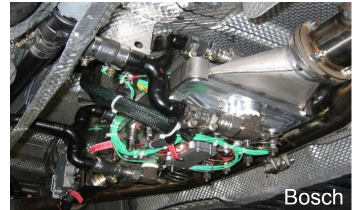
Bosch Prototype TEG in exhaust system
