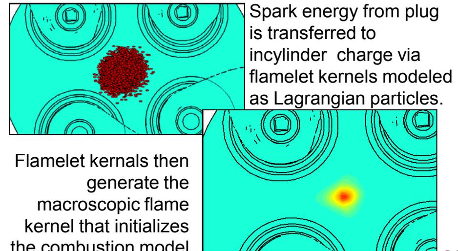
Spark energy from plug is transferred to incylinder charge via flamelet kernels modeled as Lagrangian particles.
