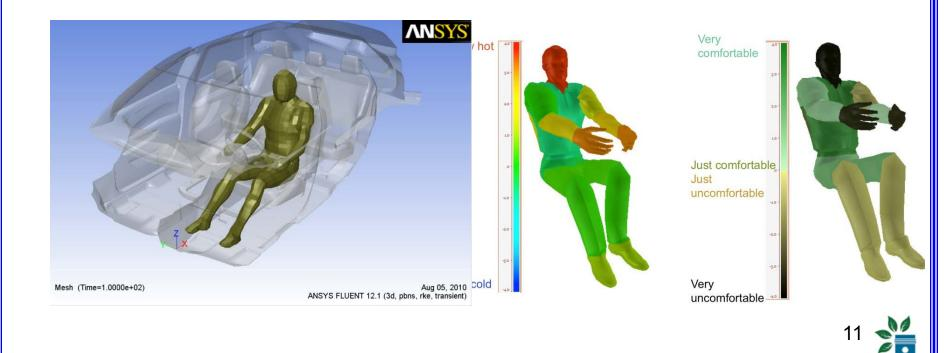
• Thermal comfort human subject testing data from UC Berkeley's environmental test chamber was used for GM's VTCE tool validation.
