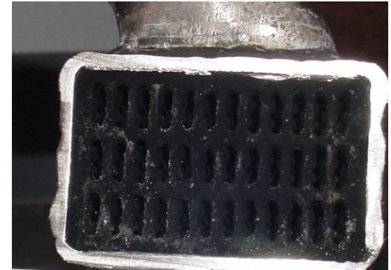
A fouled cooler in an engine test (200 hours)
