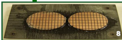
N and P Hot Pressed Pucks After Slicing
