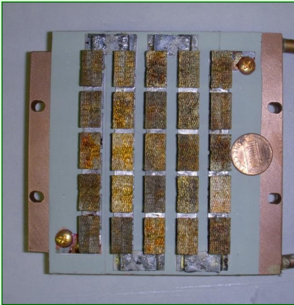
5 - 13W Modules (theoretical @ \Delta T=600C ) before Insulation
