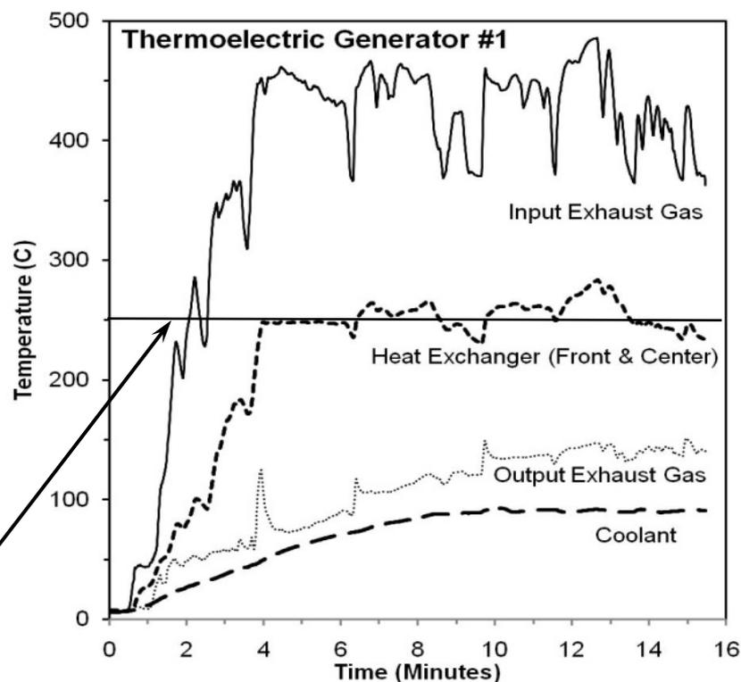
The by-pass valve set point temperature for the heat exchanger was 250°C.
