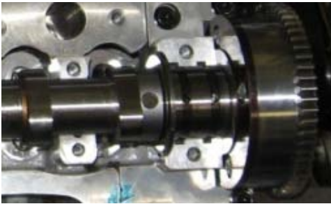
Concentric Camshafts and phaser
