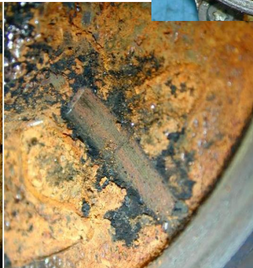
Deposit build up to 0.5mm.
