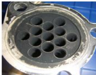
Image 12: B30 EGR Cooler Internal Aspect
