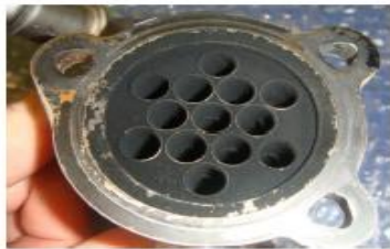
Image 10: B0 EGR Cooler Internal Aspect
