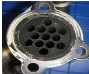
Image 11: B10 EGR Cooler Internal Aspect
