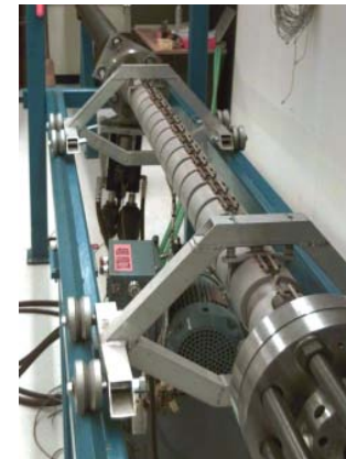
UM rapid compression facility (ign. chemistry)
