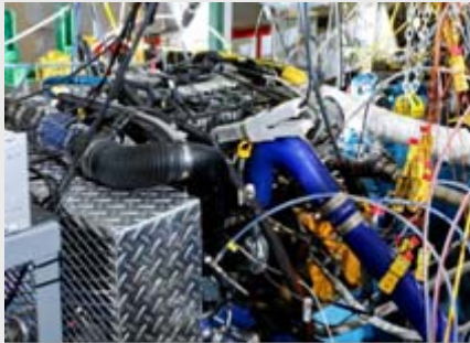
Base engine upgraded in FY 2007 to more advanced GM 1.9-L engine; increase in peak BTE for the base engine from 39% to 41%.
