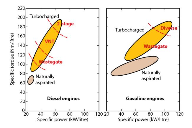
• Turbocharging is essential for modern diesel engines, and is becoming so for gasoline engines
