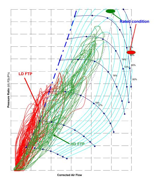
Customer driving cycle and emission cycles for light duty diesels are focused on the areas where compressors are not efficient and are close to or into surge
