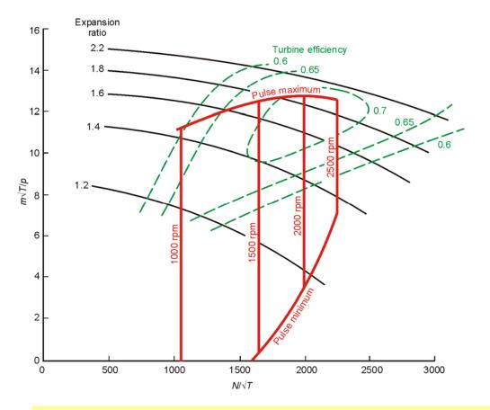
Turbine spends little time at or near its maximum efficiency during the pulse cycle
