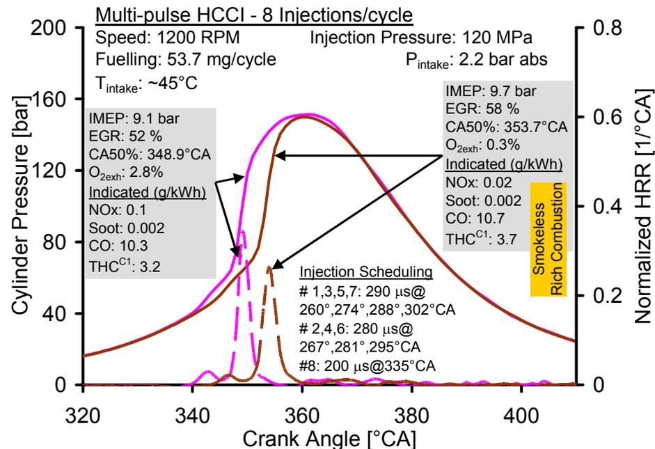
Relatively high CO & HC penalty due to large injection quantity/shot; Use of heavy EGR to improve combustion phasing
