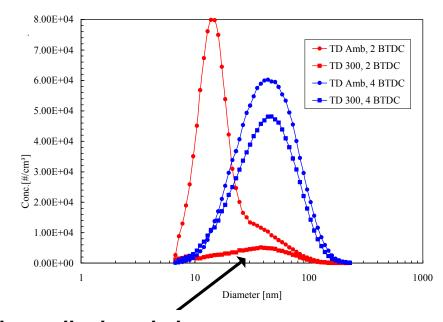
Thermally denuded particles – dry soot fraction vanishes under well chosen injection conditions
