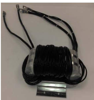
Figure 11. High frequency isolation transformer
