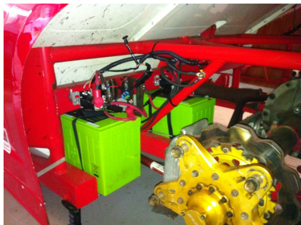
Figure 6. Li-ion battery energy storage system, driver's side, forward of driveshaft (driver's side brake shown on lower right hand side of image).
