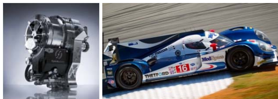
Figure 4. Flybrid system employed in #16 Dyson/Mazda at Petit Le Mans (photo by Eric Gilbert Motorsport.com)
