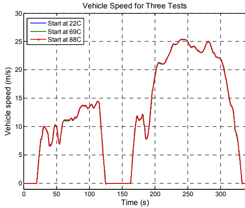
Figure 4. Vehicle speed for three selected tests. All of the test driving cases run well on UDDS.
