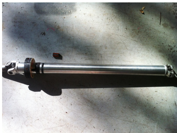
Figure 3. Drive-shaft-mounted torque sensor.
