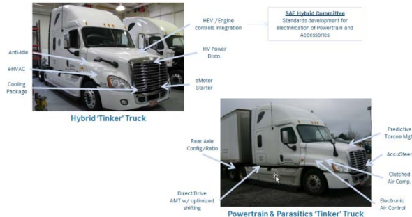
Figure 2. 'Tinker' Trucks used for functional and Fuel Economy Tests.
