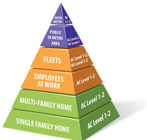
Figure 2. Depiction of the various charging levels.
