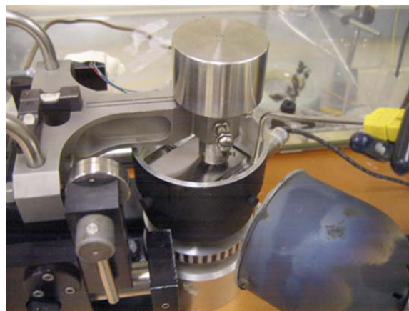
Figure 2. Pin-on-disc rig used to measure friction and wear under unidirectional sliding.
