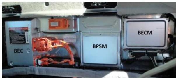
Figure 2. Schematic and Photo of the Fusion Hybrid's High-Voltage Traction Battery (HVTB).
