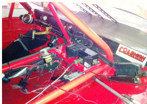
Figure 5. Data acquisition, ECU, solid-state logic-based fuse system.
