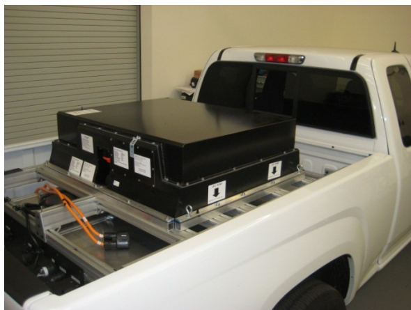
Figure 2. The vehicle bed with ESS under test (bed shell cover is removed).
