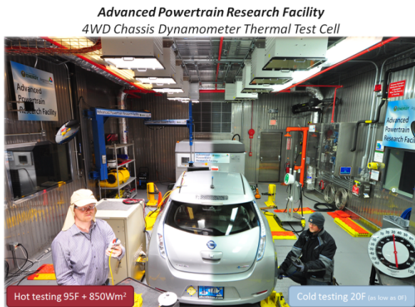
Figure 3. Nissan Leaf testing displayed at 95F with solar emulation on the left and testing at cold ambient temperature on the right.
