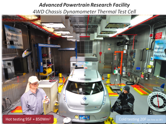
Figure 3. Nissan Leaf testing: (left) at 95°F with sun emulation and (right) at cold ambient temperature.
