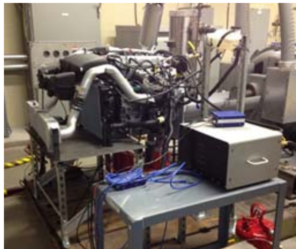
Figure 2. Ecotec LAF engine commissioned at the University of Tennessee's Advanced Powertrain Controls and System Integration (APCSI) facility.
