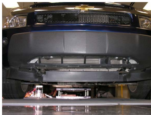
Figure 13. Equinox test vehicle with WPT coil pair.
