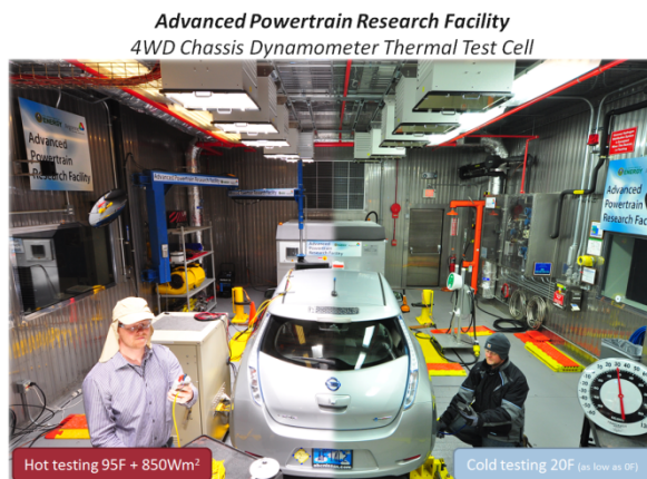
Figure 3. Illustration of testing at 95F with the sum emulation on the left and testing at cold ambient temperature.
