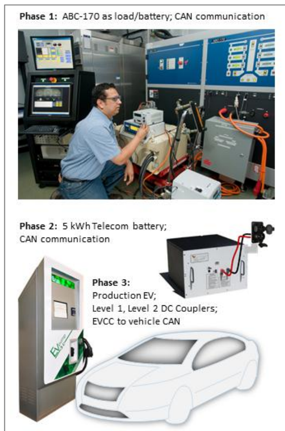
Figure 5. Test plan to verify EV-EVSE communication controllers, DC Levels 1 and 2 charging.
