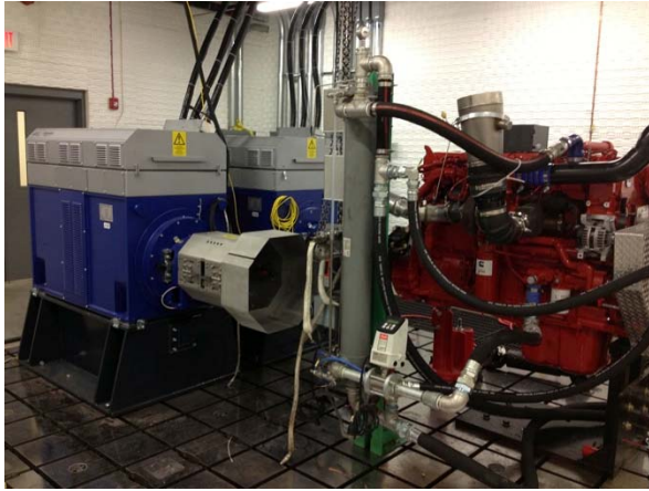
Figure 3. Current configuration of VSI Powertrain Test Cell arranged for engine-in-the-loop testing.
