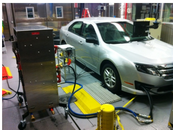
Figure 1. 2011 Ford Fusion thermal test mule and thermal conditioning cart (on left). Hoses from front grill of Fusion are engine oil inlet and outlet from the oil pan.
