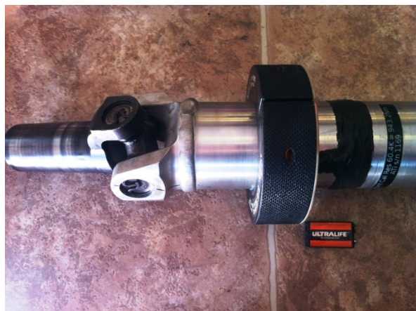
Figure 4. Torque sensor close-up. Note: System is remote powered via a 9V lithium ion battery.
