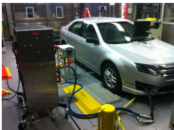
Figure 5. 2011 Ford Fusion thermal testing mule. Thermal Testing Cart shown in the lower left hand corner.
