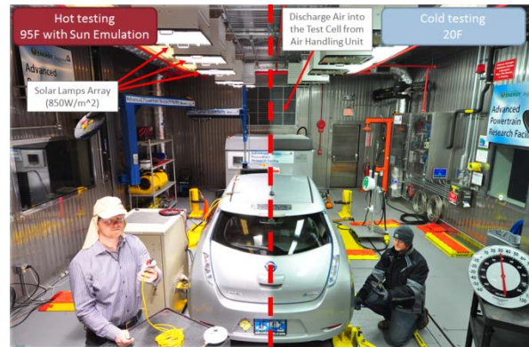
Figure 2. The thermal chamber in the APRF is able to control the ambient temperature from 20F to 95F.
