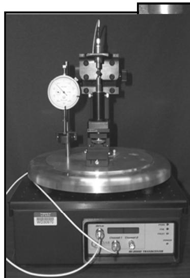
**Figure 14.** RUS equipment for structural property measurement used at PNNL. The typical sample mount between measurement transducers is shown.
