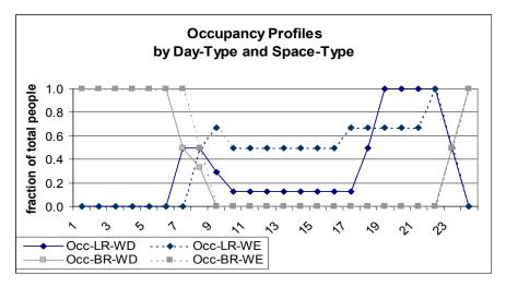
Figure 26. Detailed hourly load profiles resulting from occupants being in different parts of the house on weekdays (WD) and weekends (WE)
