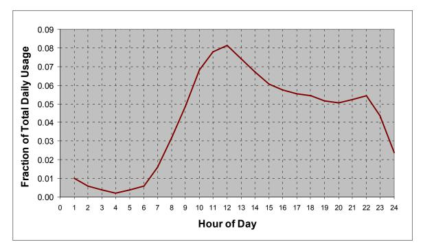
Figure 18. Clothes dryer normalized energy use profile (Pratt et al. 1989)
