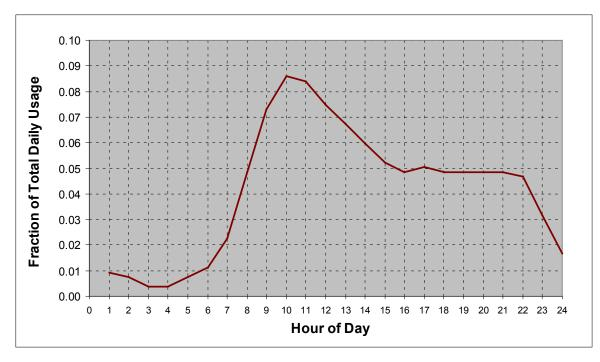
Figure 17. Clothes washer normalized machine energy use profile
