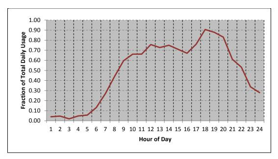
Figure 19. Common laundry clothes washer normalized energy use profile
