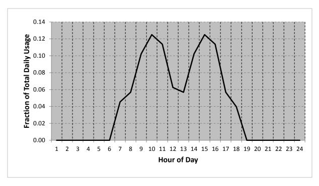
Figure 12. Central restroom sink hot water use profile
