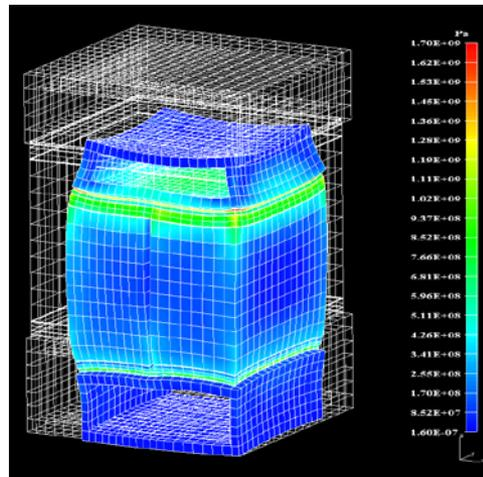
**Stresses back at room temperature after fabrication**
