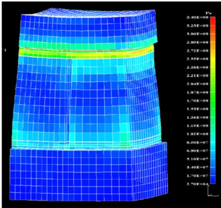
**Stresses during high temperature fabrication steps**
