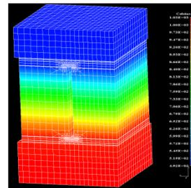
**Stresses when operating across large  $\Delta T$  Bonded to hot and cold side heat exchangers**
