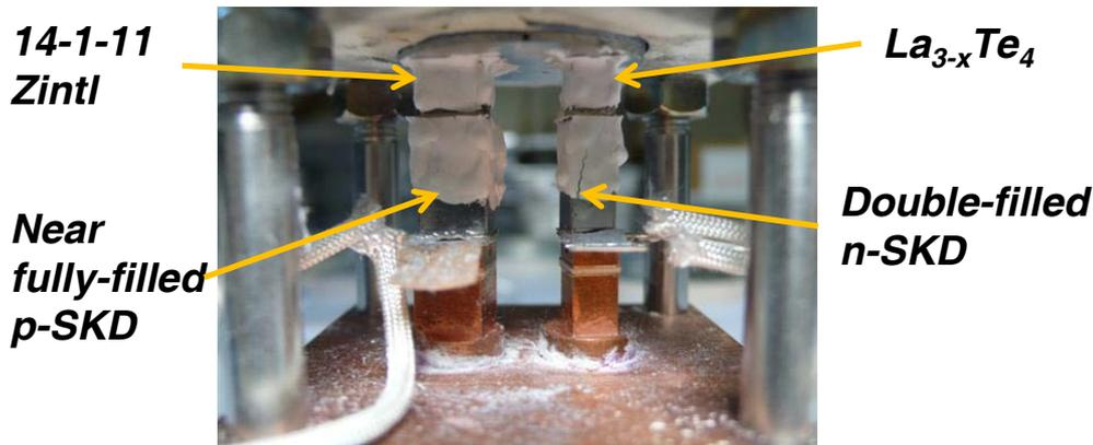
**High Temperature Segmented Zintl/ $\text{La}_{3-x}\text{Te}_4$ /SKD Couple Spring-loaded Performance Test Configuration**
