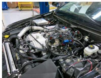
Prototype engine installed in emission and fuel economy test vehicle
