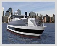
propelled by hydrogen fuel cells in a compound hybrid arrangement along with wind turbines, solar panels and a tier 2 diesel engine for additional energy needs.
