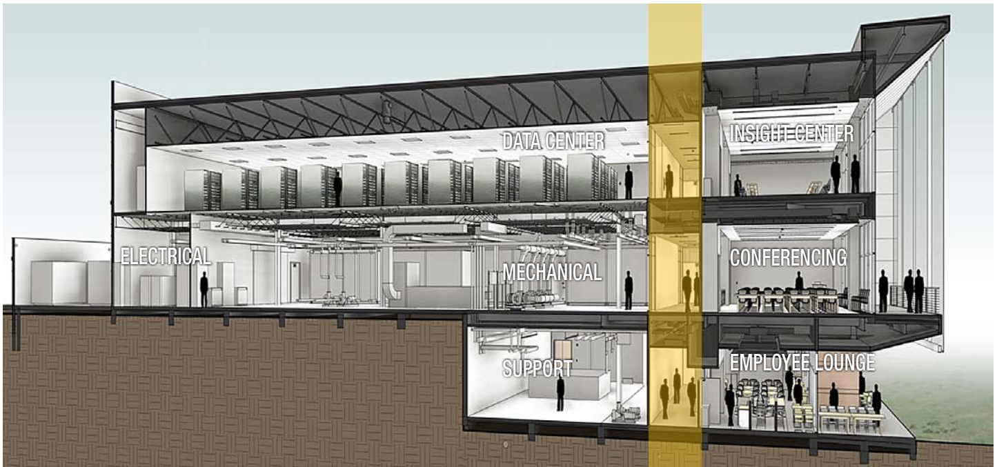
Cross section view into the ESIF HPC data center. Illustration from SmithGroupJJR
