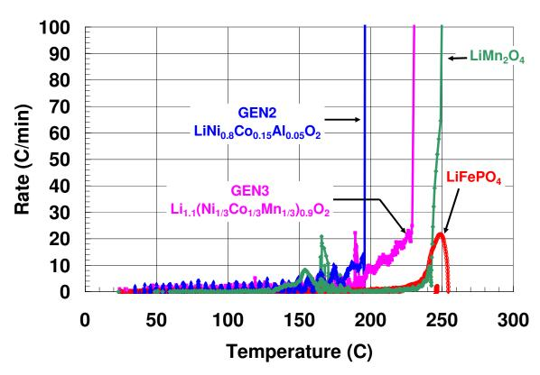
LiFePO<sub>4</sub> olivine cathodes show the greatest reduction in heating rate and increased onset temperature for runaway
