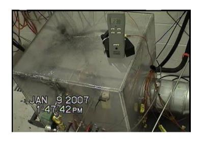
**Explosive Combustion of Vent Gases (mostly solvent vapors)**
