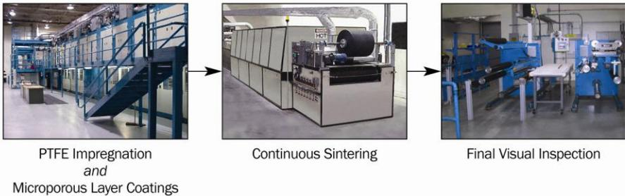
**Figure 5-9: PTFE added for hydrophobicity and microporous layer coatings added**
