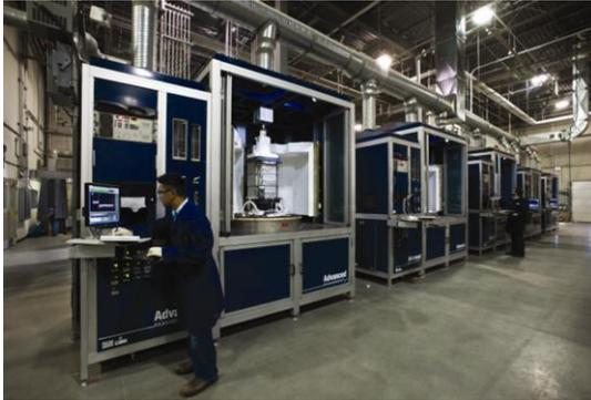
Figure III-5: Test stands for planar SOFC stack fabrication
