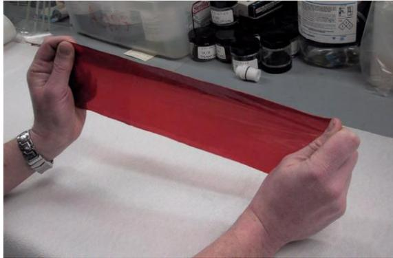
Figure 5-6: PBI sol-gel membrane
