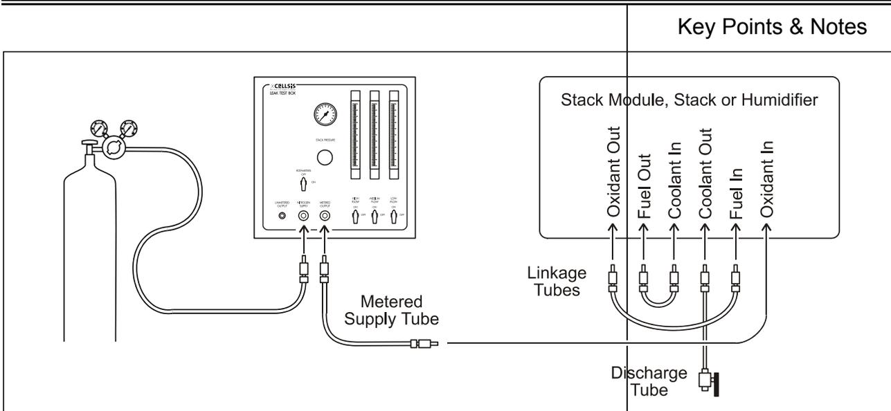
**Figure 7-25** Typical Individual Internal/External Leak Test Equipment
