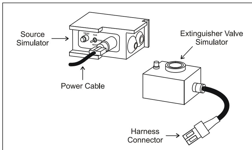
**Figure 7-43** Typical Fire Suppression System Test Equipment
