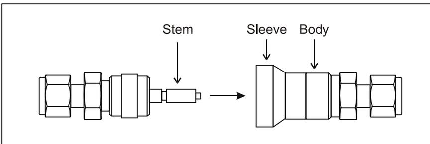
**Figure 7-4** Quick-Connect Fitting
