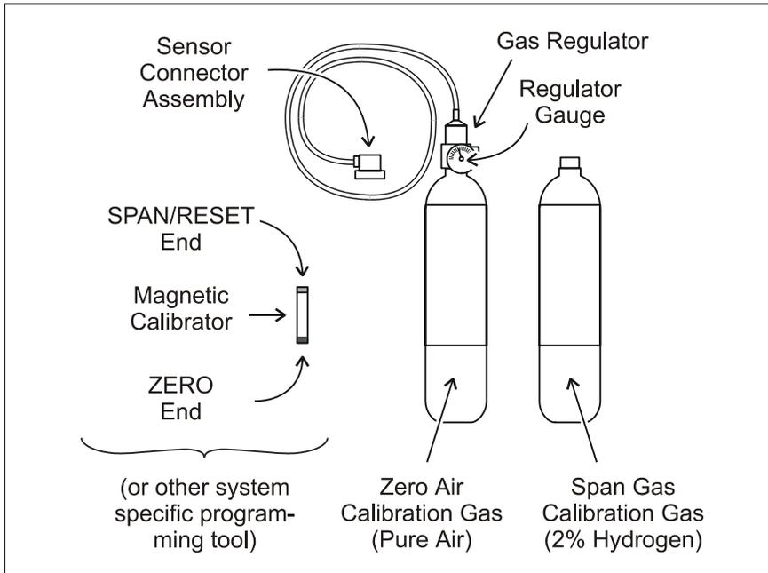
**Figure 7-39** Typical Leak Detection System Calibration Equipment
