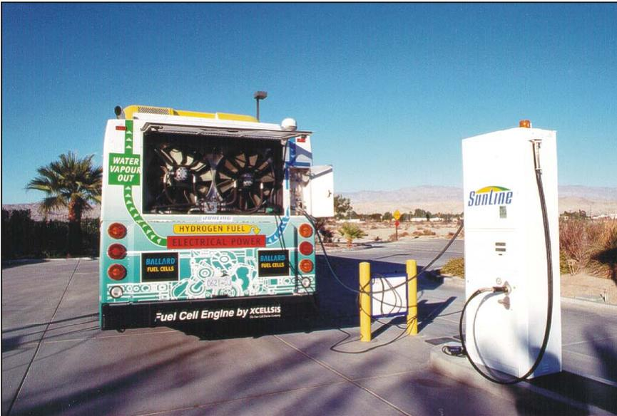
**Figure 7-9** Fueling the XCELLSiS Phase 4 Bus at SunLine Transit Agency
