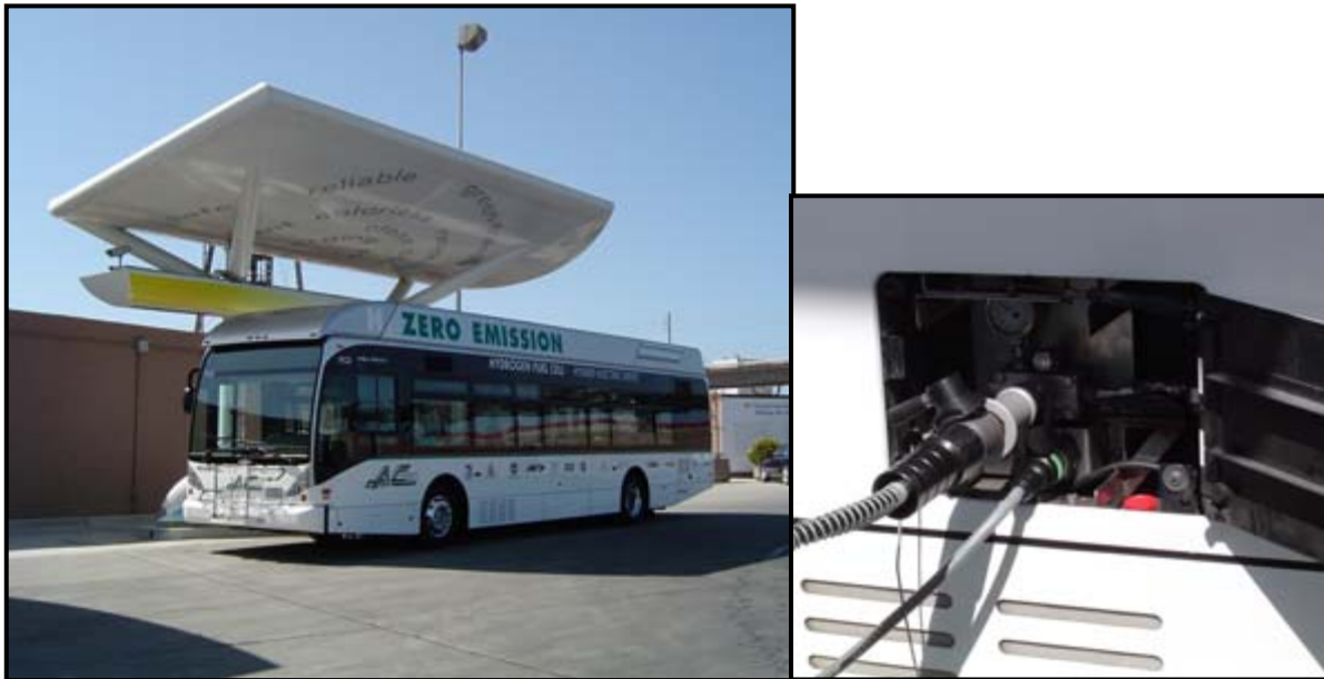
Figure 4. Fueling at the Chevron Hydrogen Station
