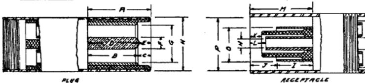
contacts must be accurately concentric to insure interchangeability.
