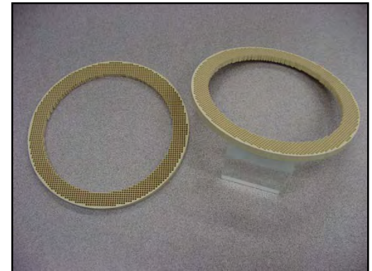
O-Ring Flexure (Diametral Compression)
