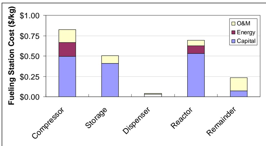
**Figure 8: Cost Breakdown for Carrier Drop-off/cH<sub>2</sub> Station**
