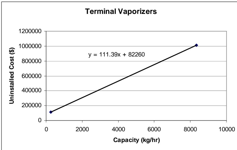
Figure 2-34 Uninstalled Costs for Terminal Hydrogen Vaporizers
