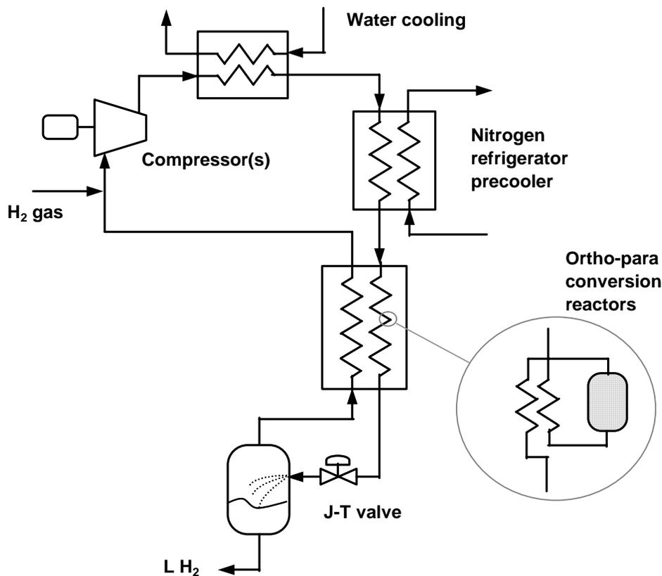
Figure 2-29 Simplified Flow Diagram for Hydrogen Liquefaction Plant
