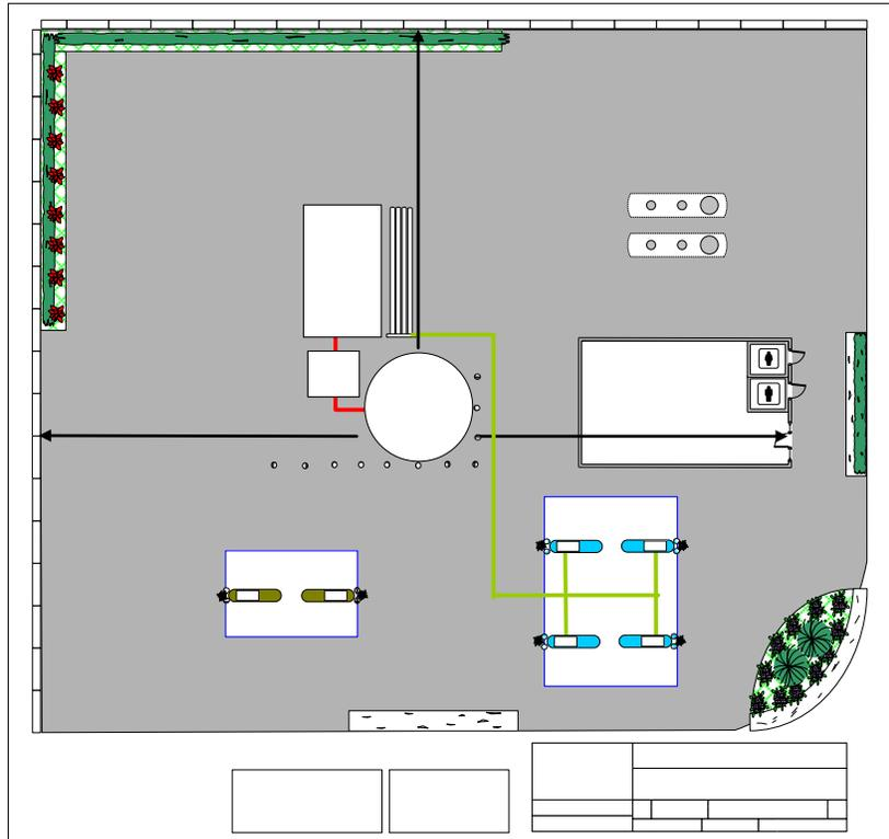
Figure 2-41 Liquid Hydrogen Supplied Fueling Site Plan
