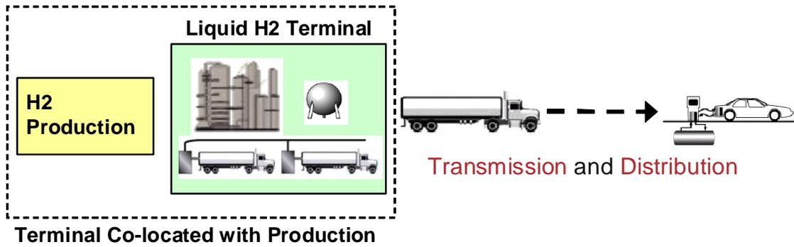
Figure 0-3 Pathway 1: Liquid Delivery Pathway with Liquid Long Term Storage
