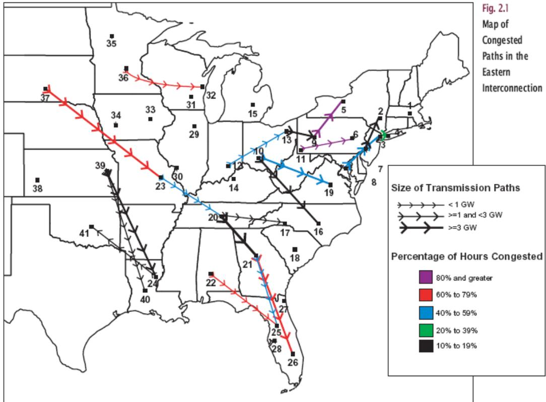
Figure 1-55 Constraint Example from the US DOE Transmission Grid Study
