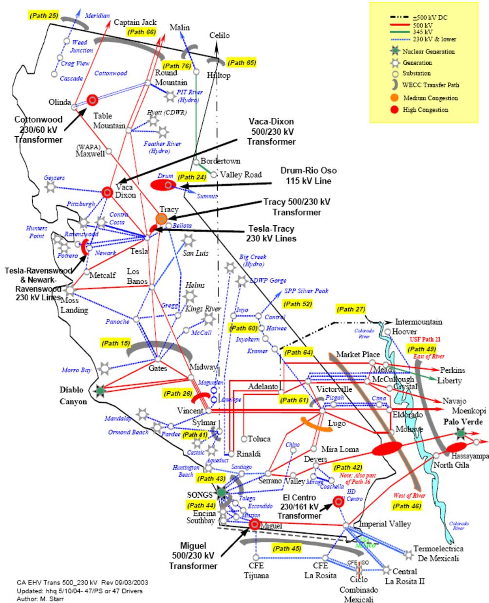
Figure 1-57 Transmission System and Constraints in California
