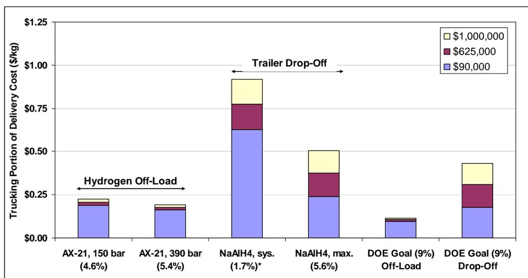
**Figure 4: Solid-State Hydrogen Trucking Cost**
