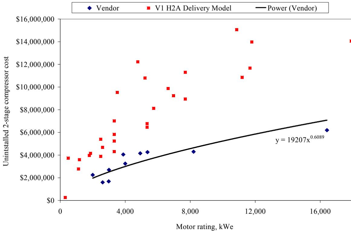
Figure 2-21 Uninstalled Costs for 2-Stage Reciprocating Compressor as a Function of Motor Rating
