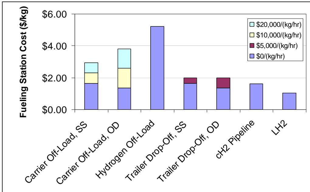
**Figure 7: Fueling Station Costs for a Variety of Delivery Options w/ Variable Costs for Discharge Reactors**
