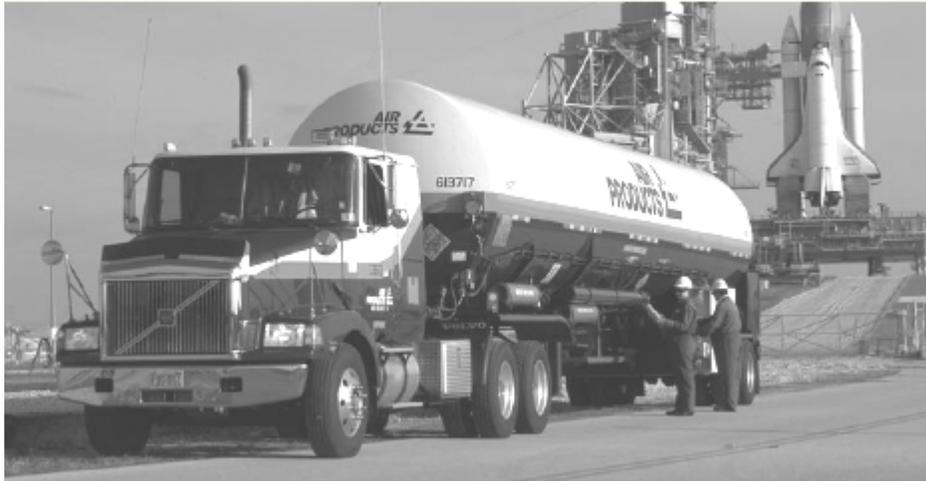
Figure 1-46 Liquid Hydrogen Transport Tanker
