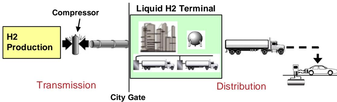
Figure 0-5 Pathway 3: Mixed Mode Liquid Delivery Pathway with Liquid Long Term Storage
