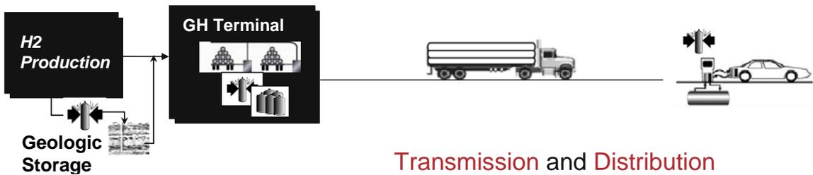
Figure 0-8 Pathway 6: Tube Trailer Delivery Pathway with Long Term Geologic Storage
