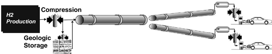
Figure 0-10 Pathway 8: Pipeline Delivery Pathway with Long Term Geologic Storage
