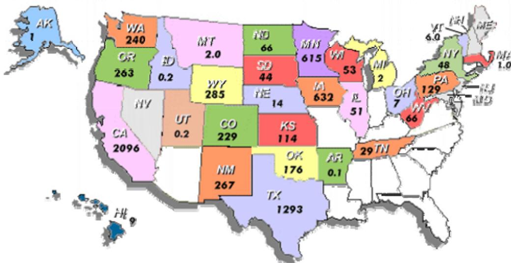
Figure 1-15 Installed Wind Generation Capacity by State, MW
