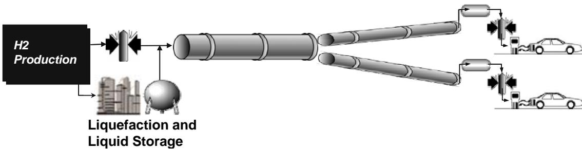
Figure 0-11 Pathway 9: Pipeline Delivery Pathway with Long Term Liquid Storage
