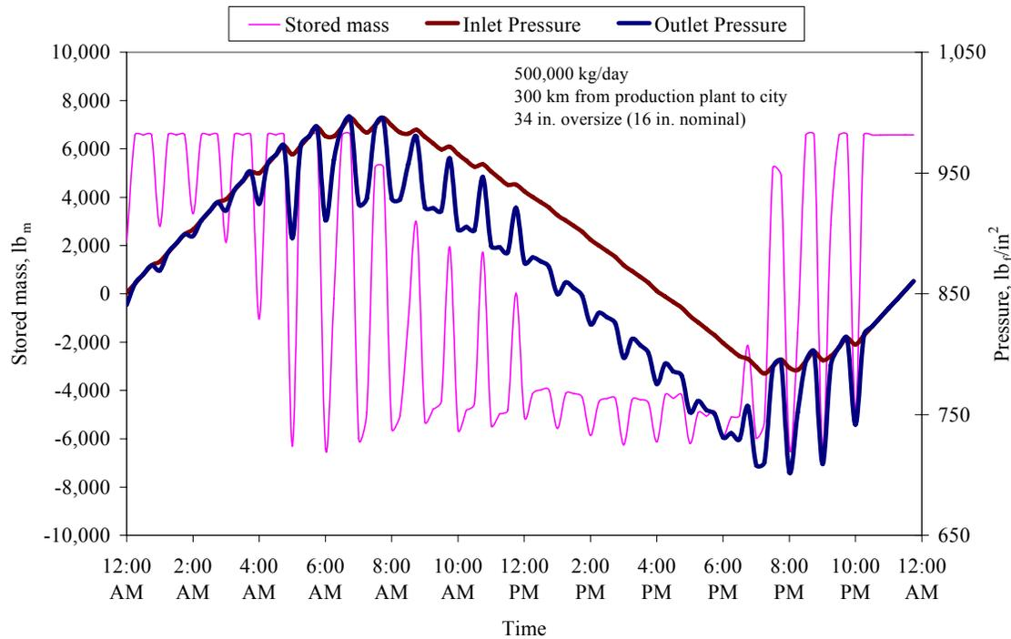
**Figure 2-46 Pressure Distribution in Oversize Transmission Pipeline**
