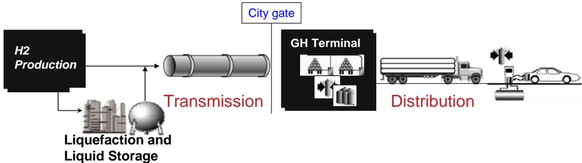
Figure 0-7 Pathway 5: Mixed Mode Tube Trailer Delivery Pathway with Liquid Long Term Storage
