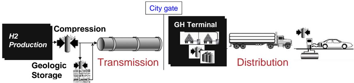
Figure 0-6 Pathway 4: Mixed Mode Tube Trailer Delivery Pathway with Long Term Geologic Storage
