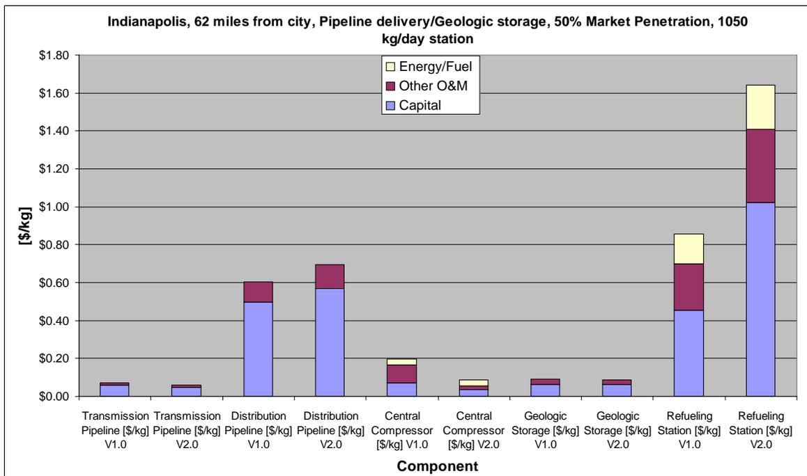
Figure 3-2 Comparison of Components' Cost Contributions in V1.0 and V2.0 of HDSAM for Pipeline Delivery Pathway
