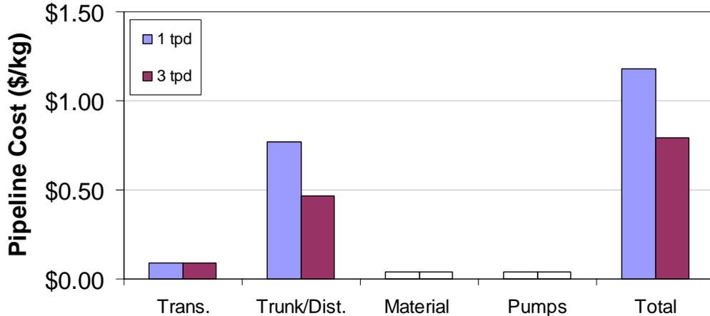
**Figure 6: Pipeline Delivery Cost Breakdown**
