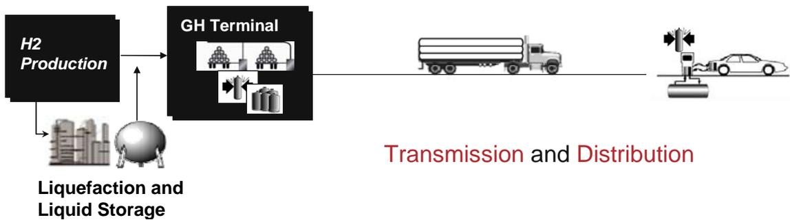
Figure 0-9 Pathway 7: Tube Trailer Delivery Pathway with Long Term Liquid Storage
