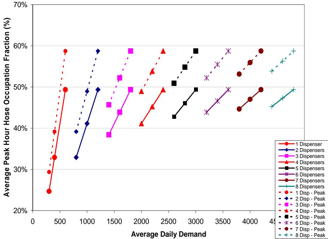
Figure 2-51 Recommended Number of Refueling Station Dispensers
