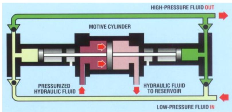
Figure 2-24 Cross Section of a Hydraulic Intensifier
