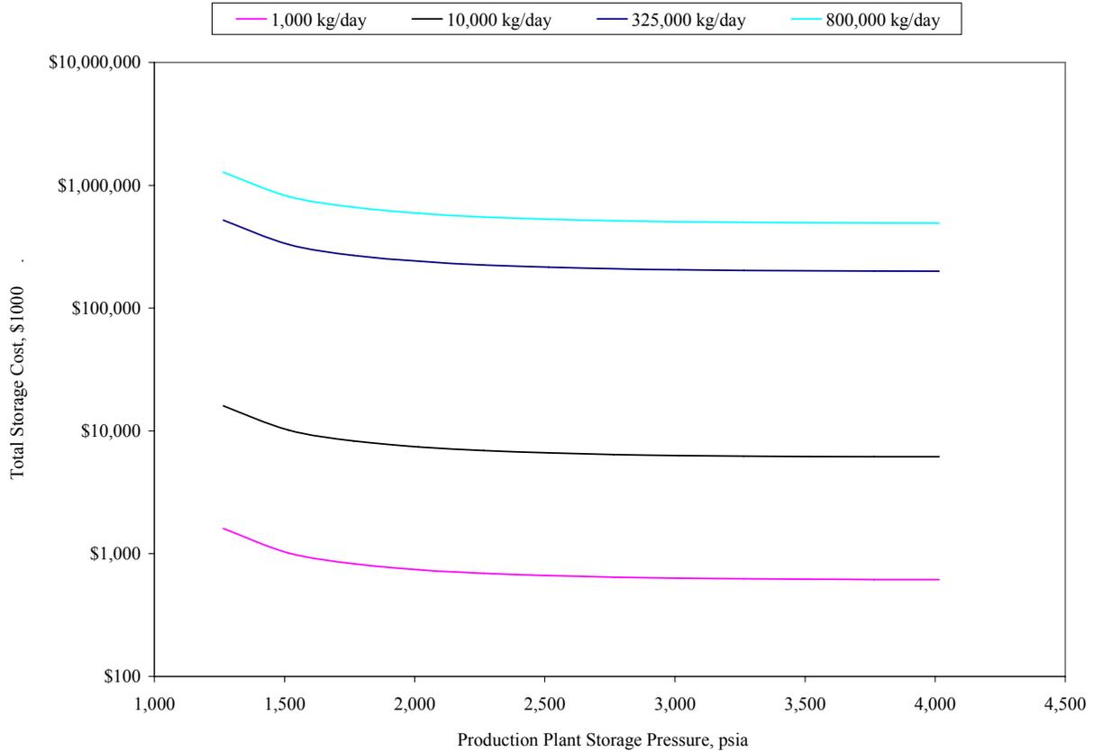
**Figure 2-15 Gas Terminal Storage Cost as a Function of Production Plant Capacity and Storage Pressure**
