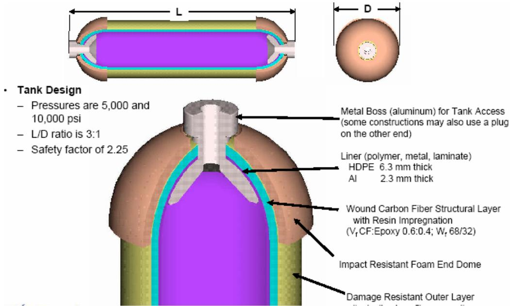
Figure 1-47 Compressed Hydrogen Composite Tank Design
